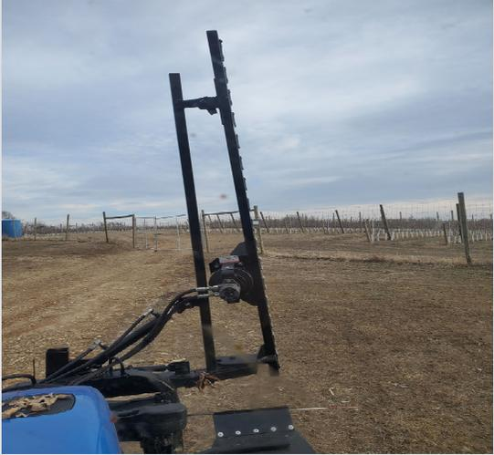
A photograph of a custom-built hedging unit mounted on a tractor. The unit consists of a vertical frame with a horizontal bar at the top, which is the sickle bar. The tractor is in a field, and the background shows a fence and a cloudy sky.
